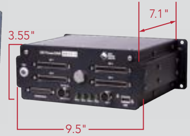
4-SLOT BRICK (DNR-BRICK) 130,000 hours
